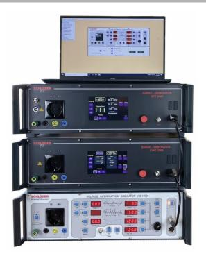
The program EMC-SOFT allows to operate the Schlöder interference generators from a PC via a serial interface or USB port (USB-RS232 converter). For this purpose, up to 9 selectable COM ports are available in the software.
